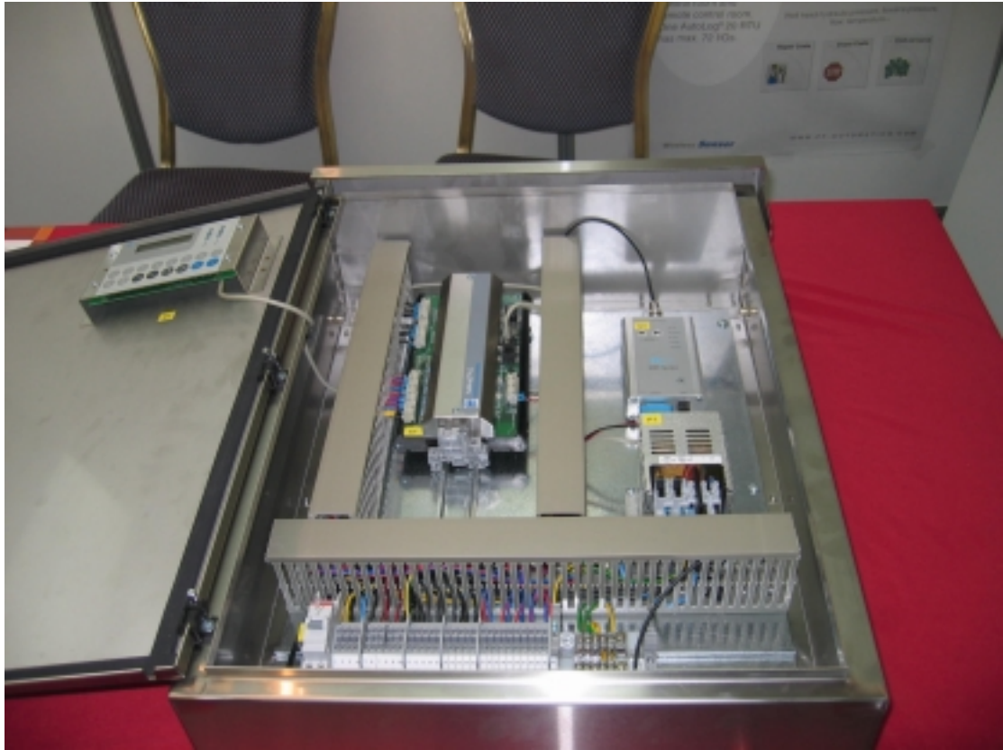
Photo above: AutoLog® Cathodic Protection (CP) RTU
