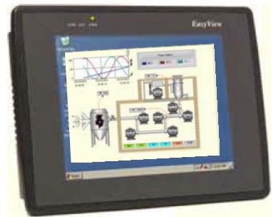
WinCE/XP 10.4" VGA TFT Touchscreen with Web Studio SCADA application
